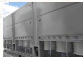
Load Bank for Shop test 2000kW x 3set /380V
