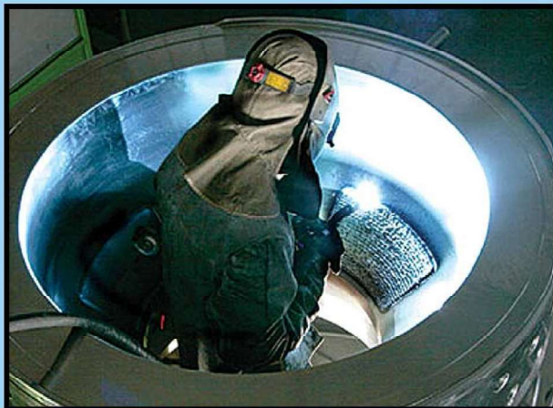
▲ INCONEL Cladding on New Cylinder Cover
