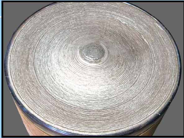
▲ INCONEL Cladding on New Piston Crown
