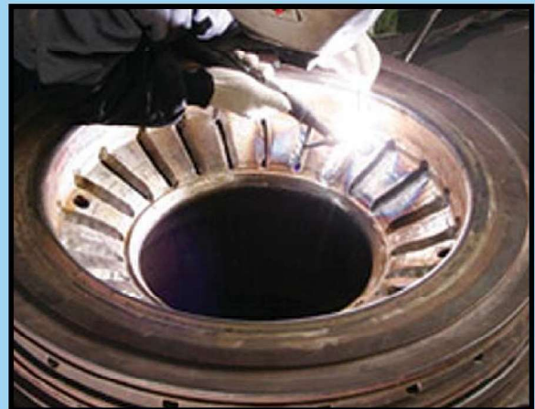
▲ GTA (Gas Tungsten Arc) Welding
