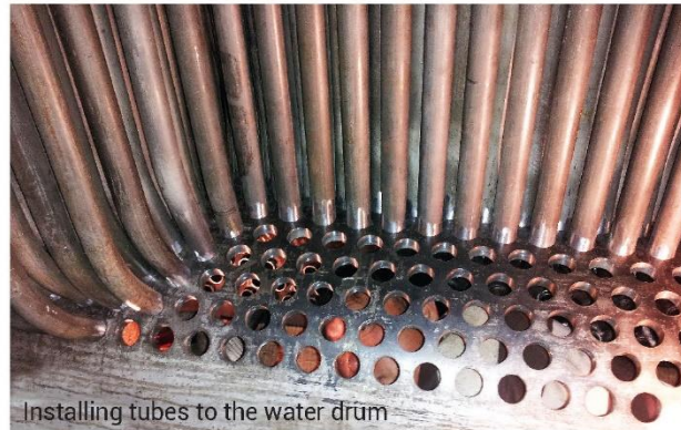
Fabricate of the steam drum & water drum
