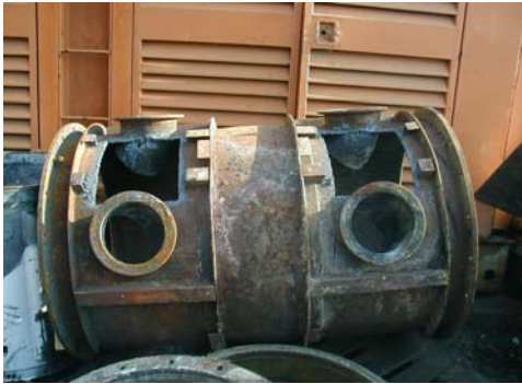
Deformed exh pipe
