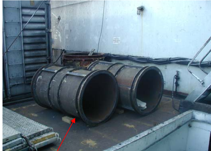
Fabricated new exhaust manifold
