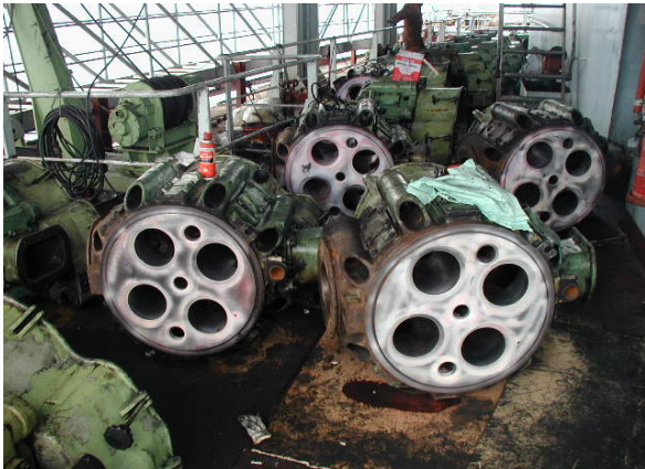
Removed Cyl., cover on deck inspection by dye check
