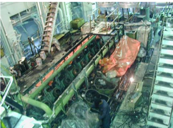
After removed exh manifold
